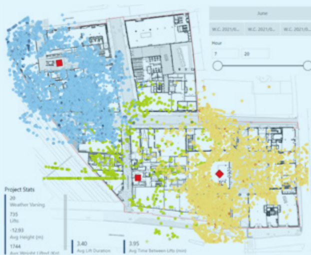
FIGURE 2 – Tower Crane interaction by operations
